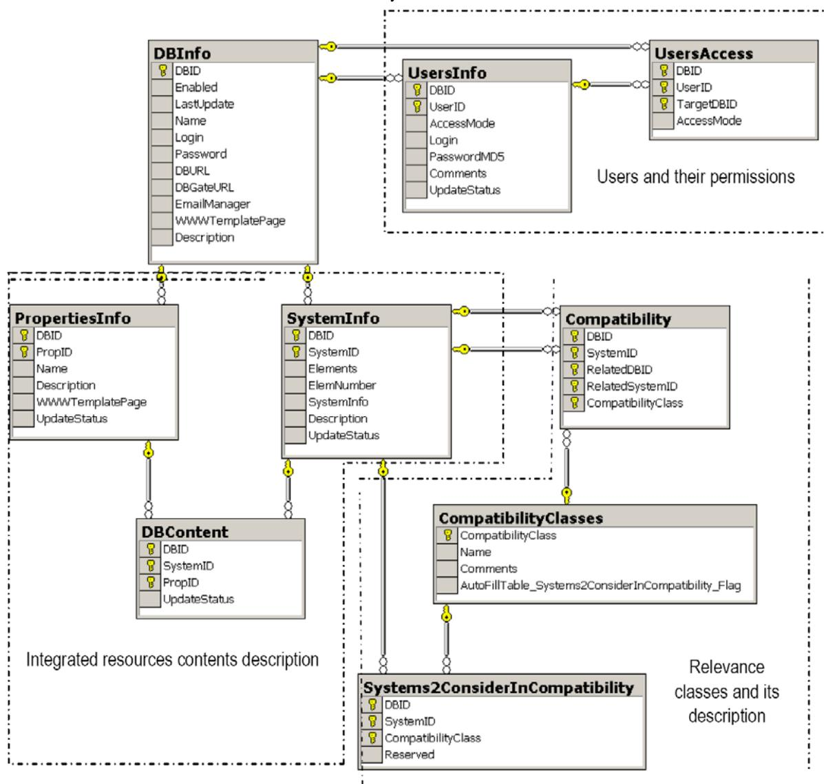
Fig. 6. Metabase structure for DBs Web-applications integration.
