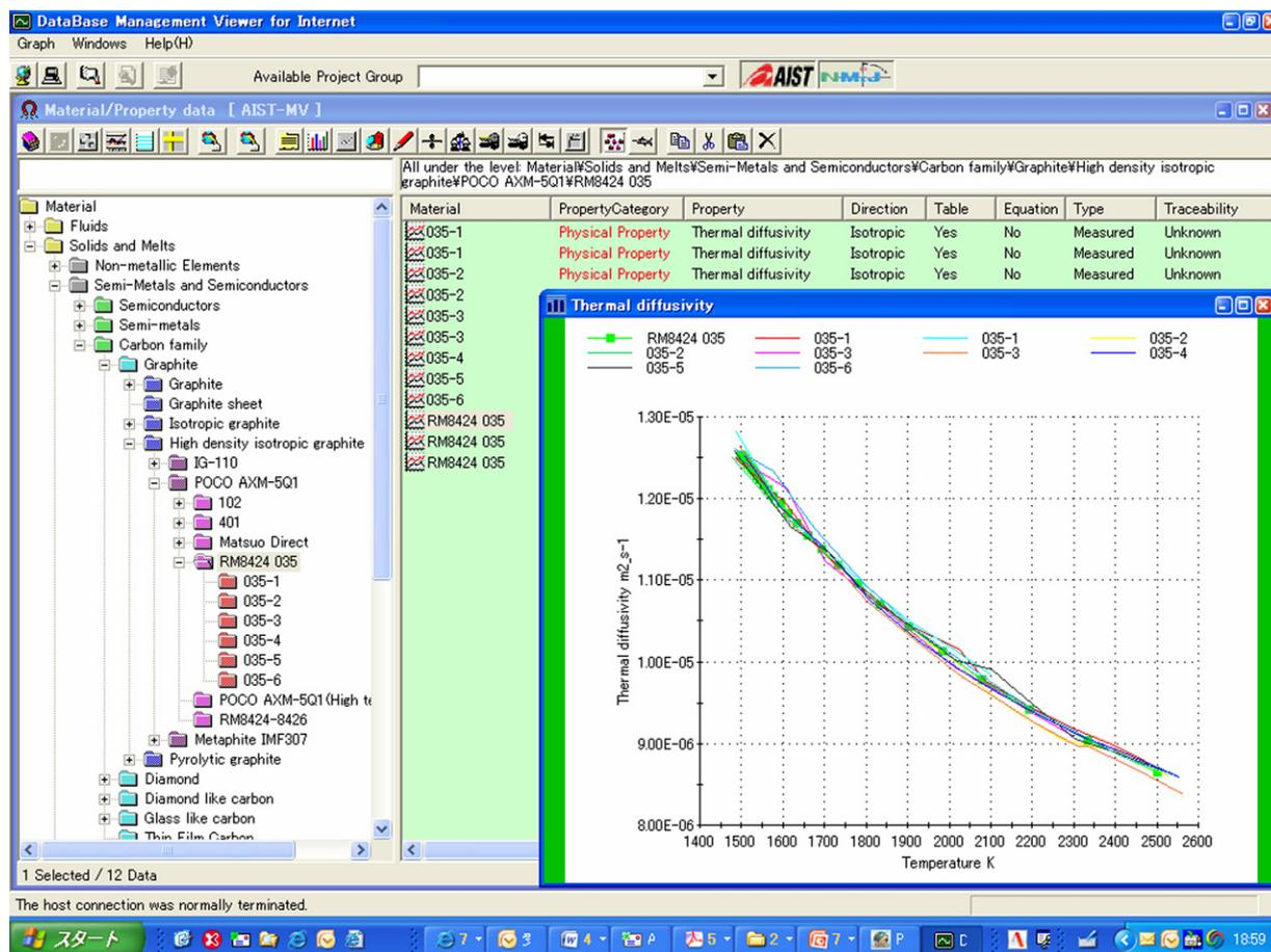
**Figure 10.** Graphical user interface of the network database for thermophysical properties. Hierarchical classification and graph are displayed for POCO AXM-5Q1 graphite.
