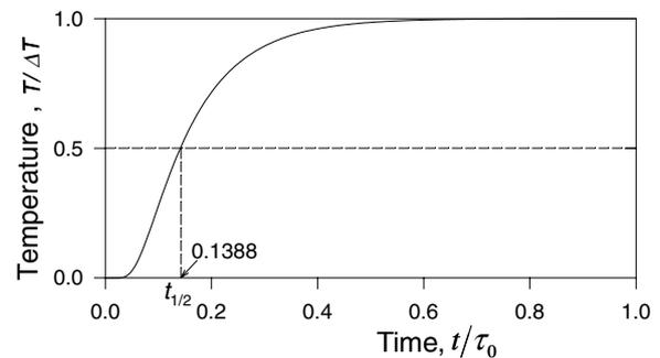
**Figure 6.** Temperature response at the rear face of the specimen after impulse heating to the front face.
