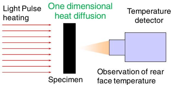
**Figure 4.** Basic configuration of the light pulse heating method for thermal diffusivity measurements.
