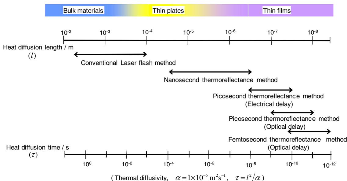
**Figure 8.** Observable heat diffusion time and observable thickness of the specimen covered with four types of light pulse heating methods with a thermal diffusivity of  $10^{-5} \text{ m}^2 \text{ s}^{-1}$ .
