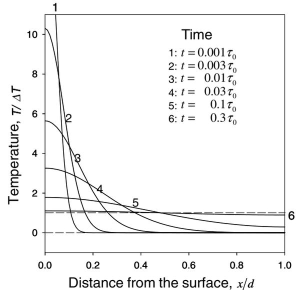
**Figure 5.** Chronological change in temperature distribution inside the specimen after impulse heating to the surface.
