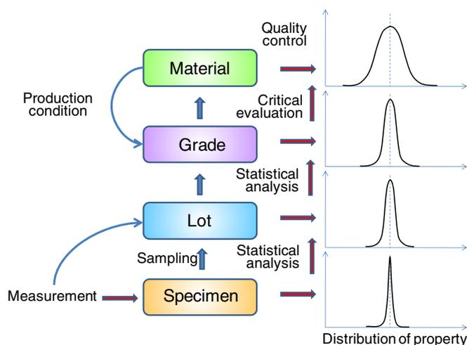
**Figure 3.** Evaluation process of material property from the measured data for specimens to lot and grade materials.
