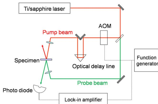
**Figure 7.** Block diagram of an ultrafast laser flash system for measuring thin film thermophysical properties by picosecond pulsed laser heating.
